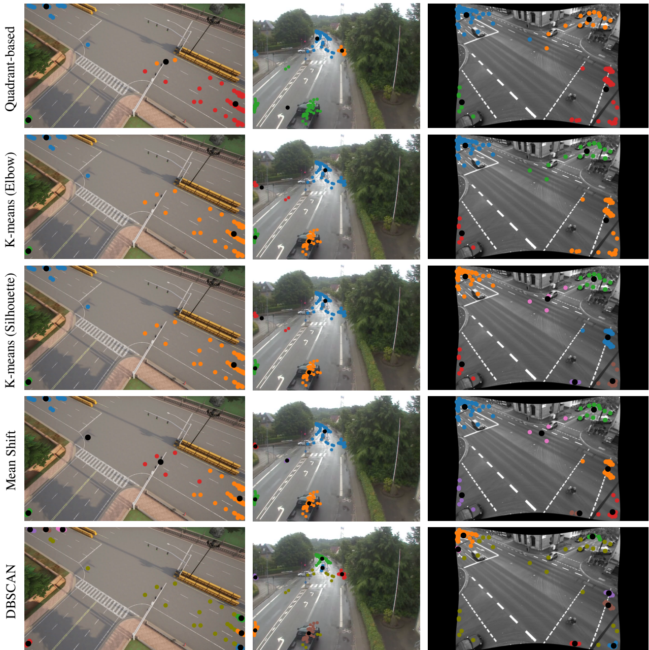
Figure 3. Samples of the first frame, where the initial and final points for each detected vehicle trajectory are overlaid on the frame. The columns, from left to right, represent the CARLA1, Hasserisvej-1, and Seq1_SK_1 videos, respectively. Each row corresponds to a different clustering method. Points that belong to the same cluster (as determined by the clustering method) are shown in the same color, while cluster centroids are marked in black.
