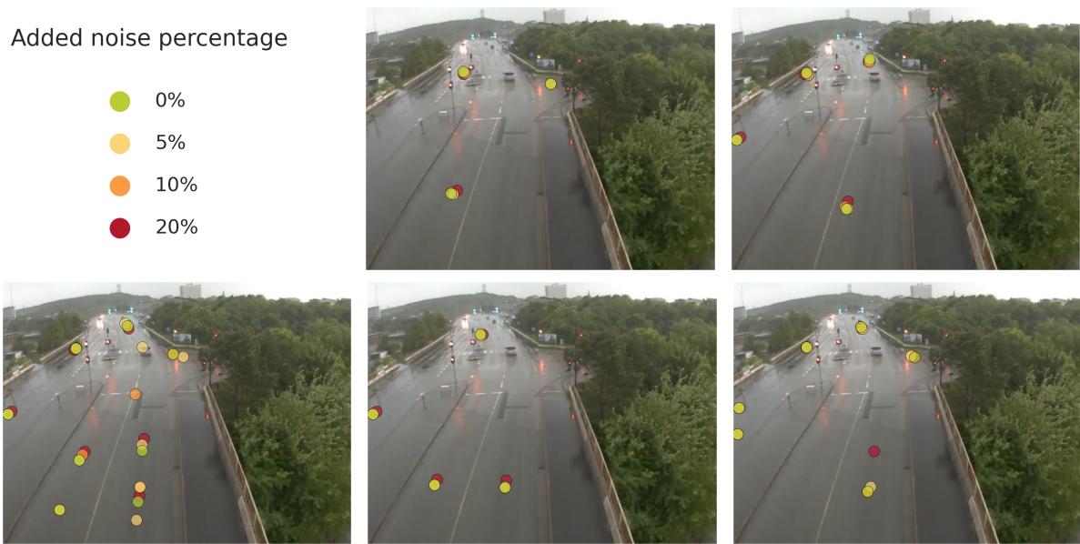
Figure 6. Samples of the first frame from Ostre-3 video, where the cluster centroids for each percentage of added noise are overlaid on the frame. From left to right and top to bottom, correspond to the legend: Quadrant-based, K-means (Elbow), K-means (Silhouette), Mean Shift, and DBSCAN.
