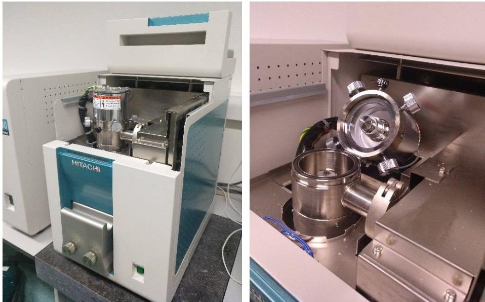
Fig. M3. Left. Main unit of the scanning electronic microscope Hitachi TM-1000. Right. Detail of the electron column.
