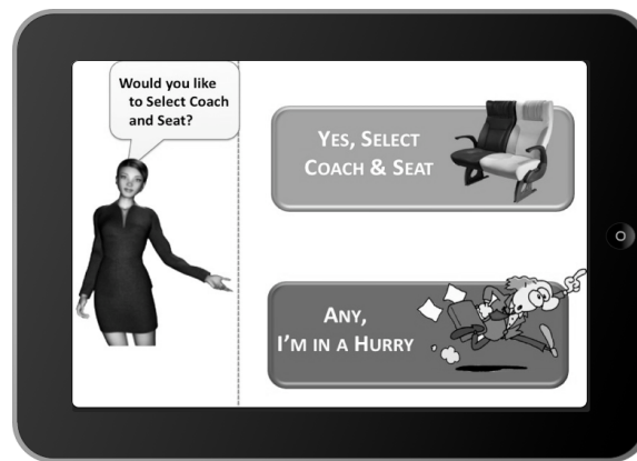
Fig. 5.5 The second iteration of the prototype of AGILE interface for the train ticket transaction, shown in an iPad2. Note the absence of Goals and Steps maps. There still remain the virtual agent (assistive area) and the region with buttons (interactive area)
