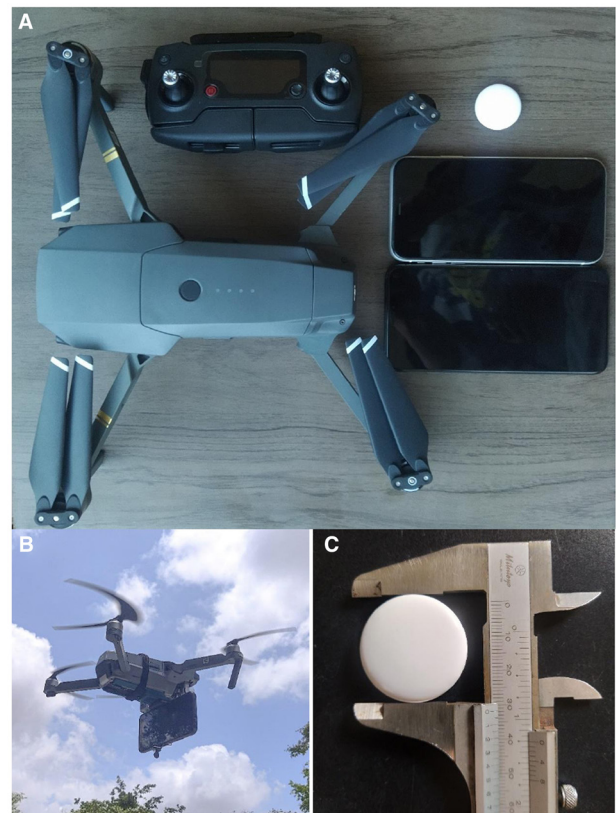
Figure 1. Off-the-shelf tracking system and components. (A) Off-the-shelf tracking system (Mavic Pro drone with controller, Iphone 8 and 11, one AirTag). (B) Mount support for Iphone. (C) AirTag.
