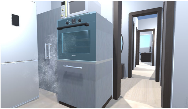
Fig. 4 Using the GADEN plugin for Unity, the gas and wind simulations can be played back in the same simulation environment the Robot@VirtualHome dataset uses. This option also offers more realistic ways to visualize the gas plume, further enabling the testing of vision-related techniques
