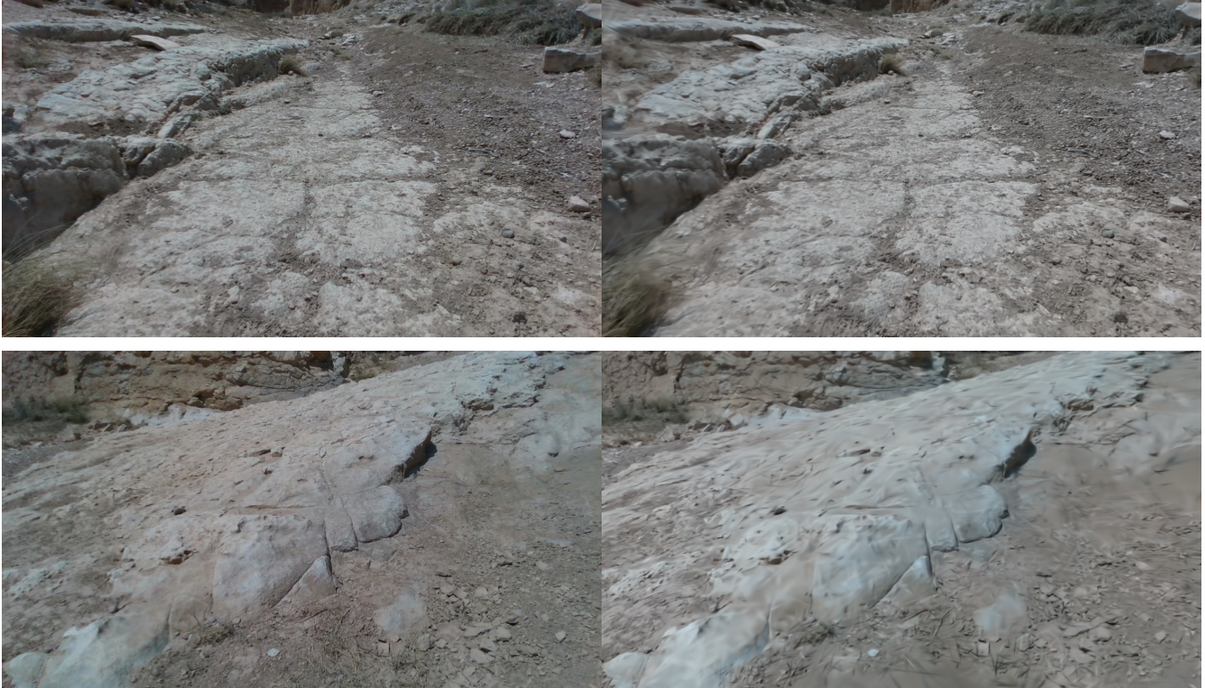
Fig. 3. Comparative examples between real-world views (left) and their corresponding 3D reconstructions (right). The visual alignment demonstrates the high geometric and radiometric consistency achieved by the proposed workflow.
