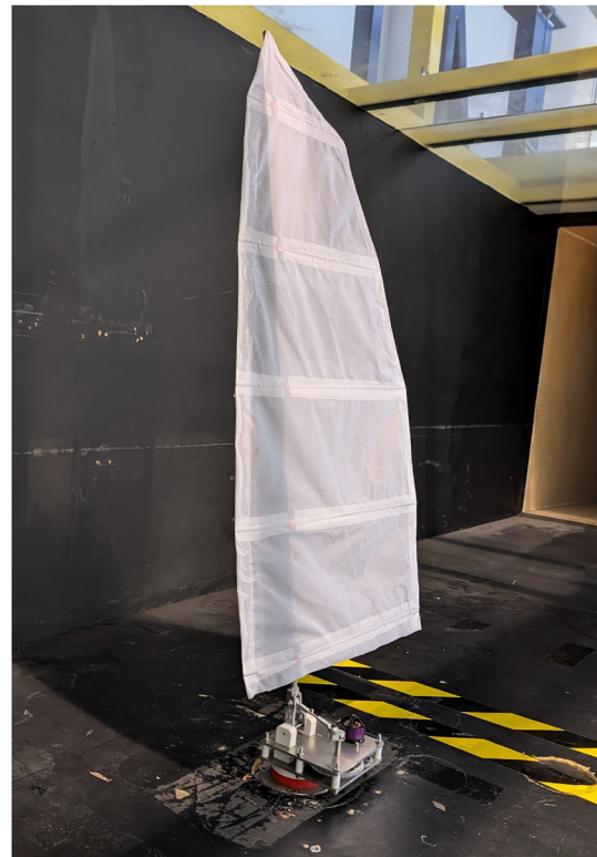
FIG. 4. Flapping mechanism fixed in the wind tunnel. Multimedia available online.
