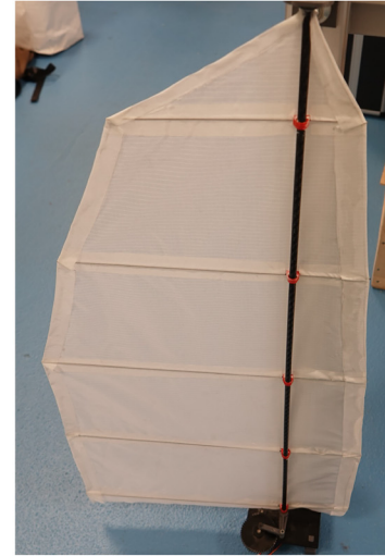
(b) Image of the testbench with the wing fixed to an aluminum structure to avoid vibrations.
