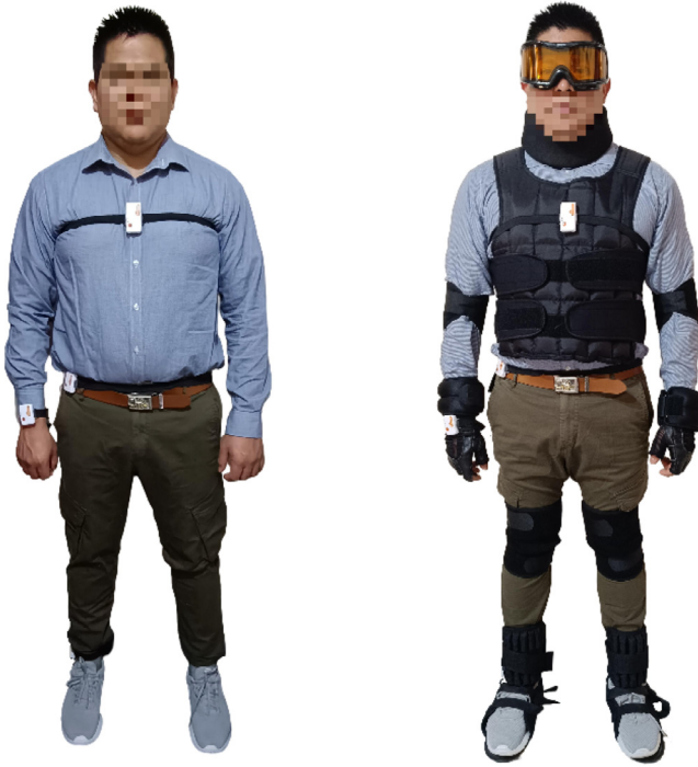
Fig. 4. Participant with the four sensing units attached to the measuring points on his body. Left image: without GERT simulator, right image: wearing the GERT simulator.
