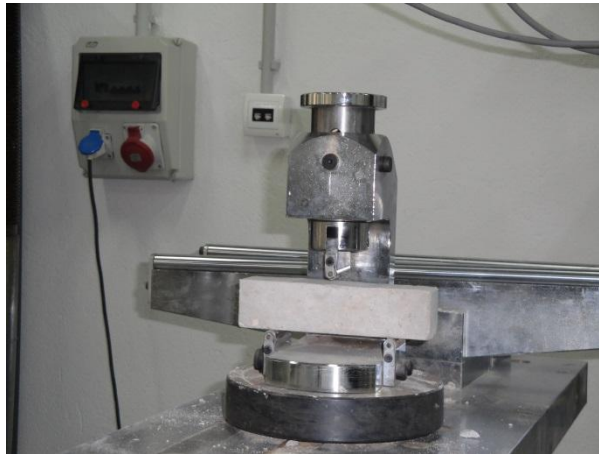
Figure 10 Charging device used in the test specimens (central point)
