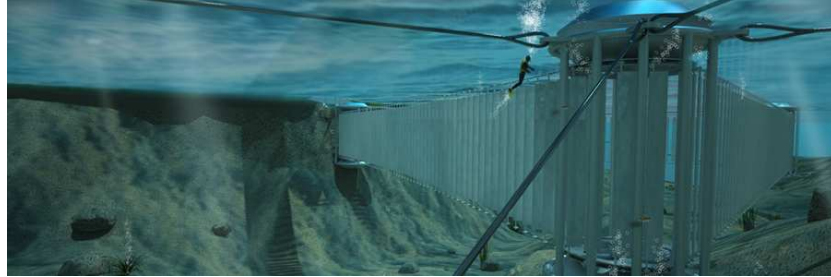
Figure 1.1: Sketch of the design of flat plate cascade (TidalSail S.A., 2014).
