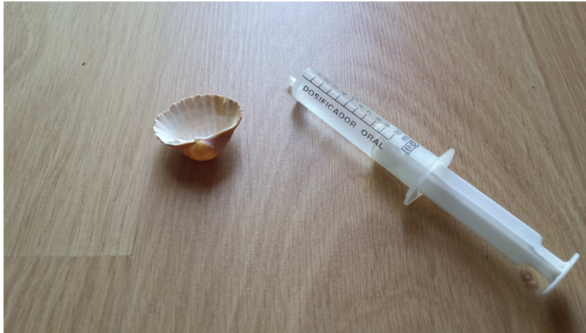
Figure 3.15: Method to calculate the volume of the seashell cavity.
