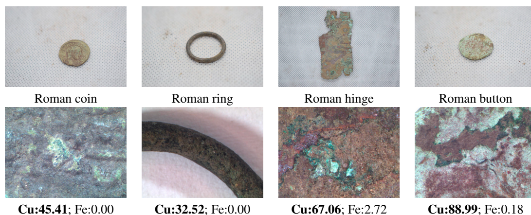
Fig. 2. Sample of bronze artefacts with one associated microscopy image and XRF-derived chemical composition in terms Cu. The concentration of Cu is highlighted in bold.
