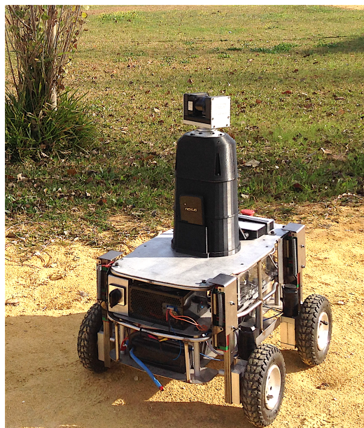
Fig. 1. Andabata mobile robot with its 3D laser scanner on top.
