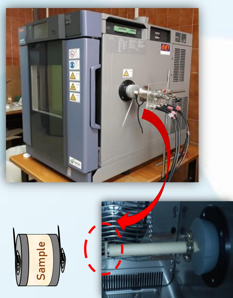
Humidity chamber (Espec SH-222) for proton conductivity measurements (UMA).
