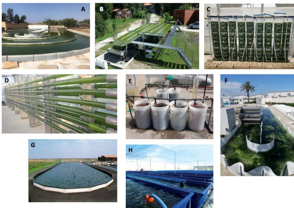
Figure I. 12. In land facilities for micro- and macroalgae cultures: MICROALGAE: A) Out door race way (UAL, Almeria), B) Thin layer cascade (Algatech, Czech Republic), C) Vertical bags (IBYDA, UMA), D) Tubular photobioreactors (IBYDA, UMA); MACROALGAE: E) In door polyethyle tanks (BEA, ULPGC), F) Outdoor raceway (IBYDA, UMA), G) Large scale raceway (Israel), H) Tanks (Ensenada, México)
