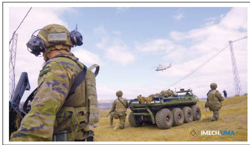
FIGURE 3. Autonomous victim evacuation: after executing the planned path, the UGV reaches the extraction point and waits for the helicopter [11].
