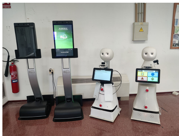
Fig. 1 The Socially Assistive Robots employed in this study. The GoBe robots are on the left, the CLARA robots on the right
