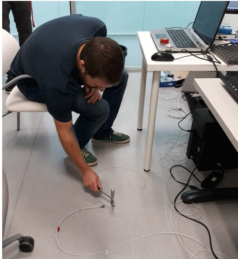
Figure A.7.: Photo showing Sergio Postigo performing the mechanical mode analysis of the old setup. The hammer is used to excite the present mechanical modes measured by the acceleration sensors (connected to the white cables).
