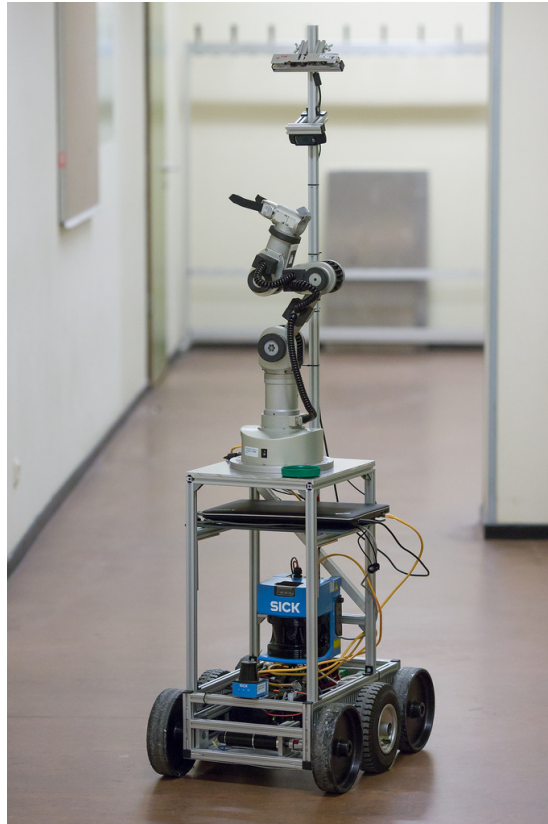
Figure 10: The robot used to record the data set, equipped with an ASUS Xtion Pro Live RGB-D camera (top) that was removed from its casing and a pair of laser scanners for localization, navigation and obstacle avoidance.
