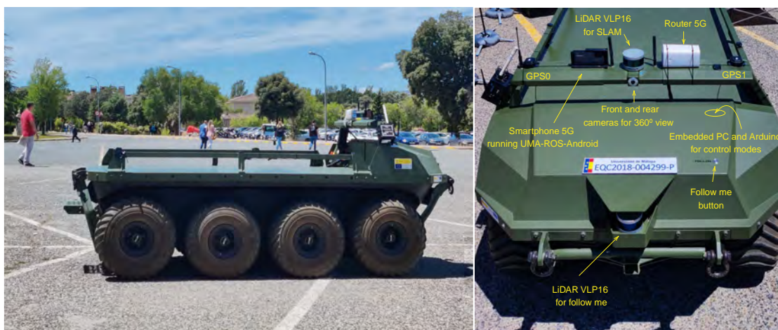
Figure 5.7 UGV Rover J8 in the experimental urban area (left) and onboard sensors (right)
