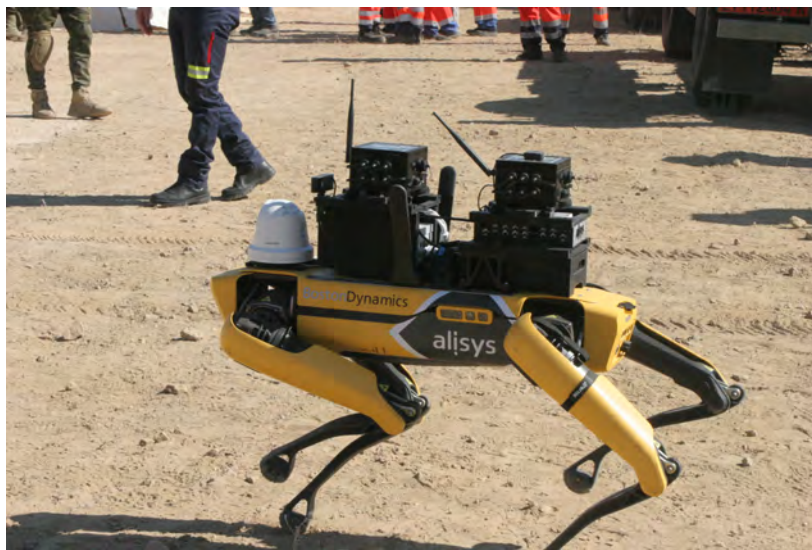
Figure A.7 Spot (Boston Dynamics) being tele-operated while carrying a LoRa sensory group
