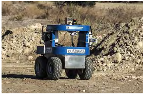
(a) Cuadriga being tele-operated while carrying a LoRa SG and a BLE scanner
