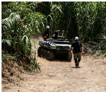
(c) Rover J8 in follow-me mode with LoRa SGs and a smartphone as part of its payload
