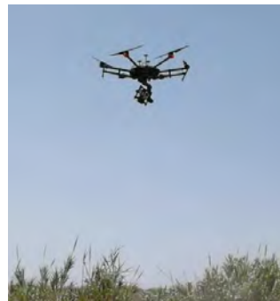
(d) DJI Matrice 600 with a smartphone as a payload on its gimbal mechanism
