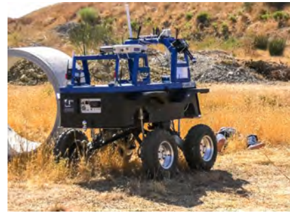
(b) Rambler close to a victim after performing a path-planning with a LoRa CN embarked
