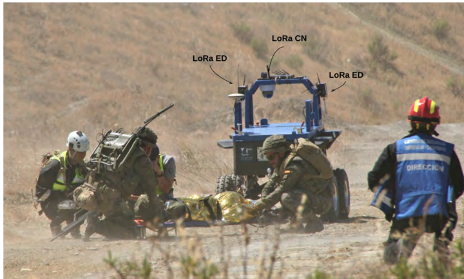
Figure 3.22 Rambler embarking LoRa EDs and CN in a ROUD scenario
