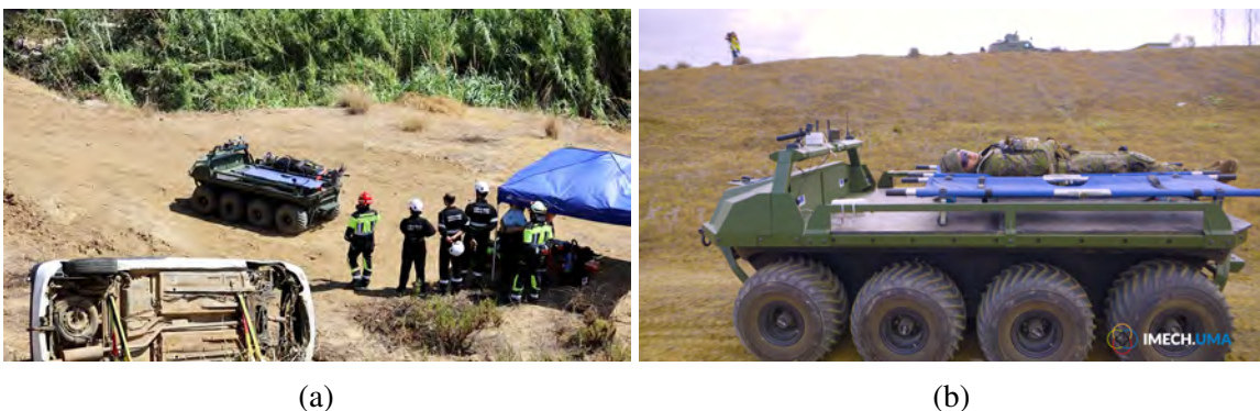
Figure A.3 Rover J8 acting as an evacuation platform.
