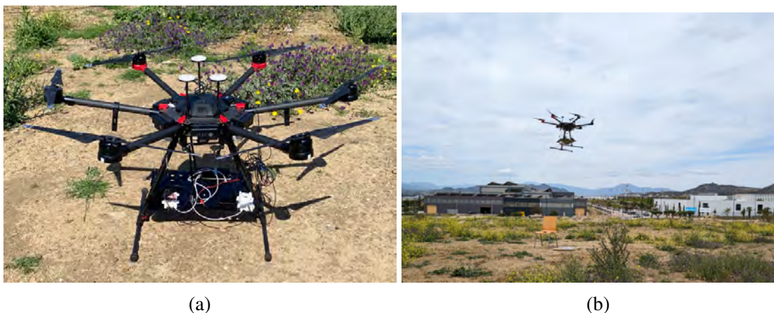
Figure A.4 DJI Matrice 600 carrying an ad-hoc 5G sensor
