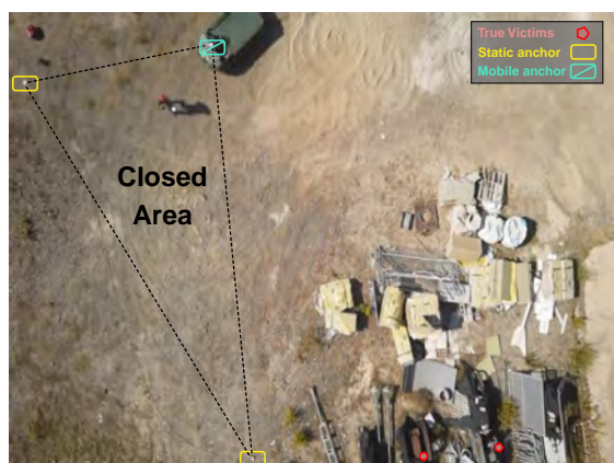
Figure 4.19 Field of view of the UAV when hovering 21 m above the UGV.
