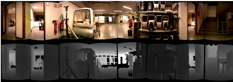
Figure 5.4: Omnidirectional RGB and depth images acquired by our RGB-D camera rig.
