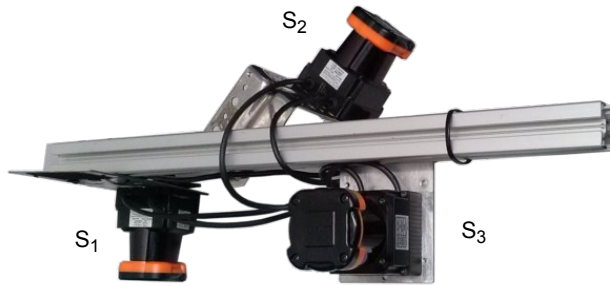
Figure 2.12: Test LRF rig with three Hokuyo UTM-30LX.
