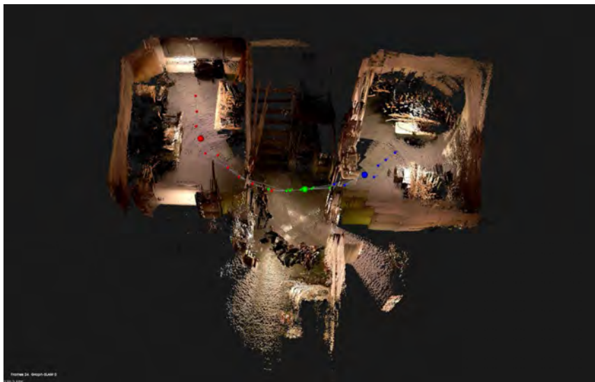
Figure 5.10: Keyframe-map of an office environment. The spheres represent the location where the keyframes were taken. The large spheres are the most representative keyframes of each local map, where different colours are used to represent such local maps.
