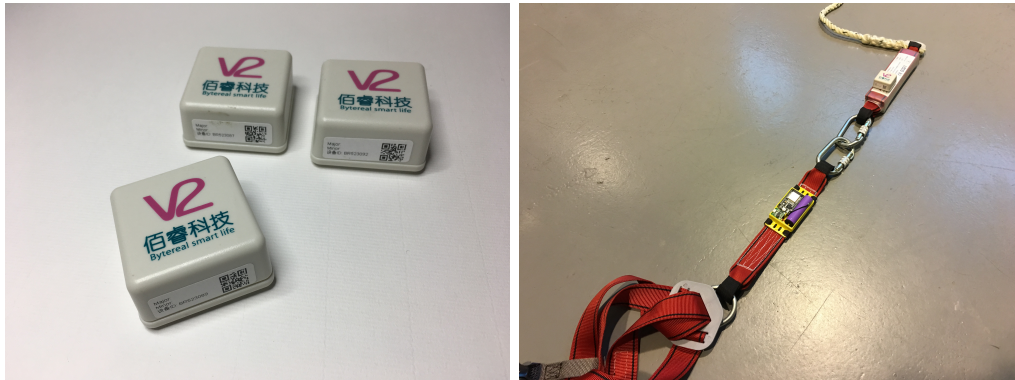
Figure 3: BLE Beacons used in the experiments and a view of the circuit (Left). The receiver (right) is based on an ESP32 chip from Espressif, with Wi-Fi and Bluetooth communications, and powered with a 18650 Li-ion battery. The detection of the lifeline attachment is possible thanks to a commercial BLE beacon placed near the carabiner.
