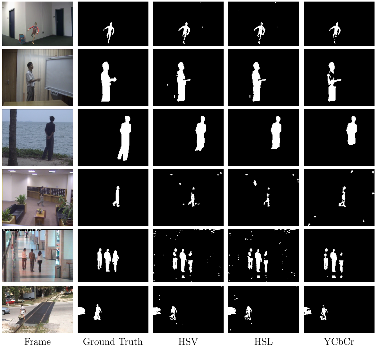
Figure 6: Foreground detection results of the GHNF model for HSV, HSL and YCbCr color spaces. Rows from top to bottom: Video2 (frame 526), Meeting Room (frame 23242), WaterSurface (frame 1577), Lobby (frame 2265), OneShopOneWait1cor (frame 375), and LevelCrossing (frame 386). The first two columns show the original frame and Ground Truth, respectively. The last three columns show the corresponding tested color spaces.
