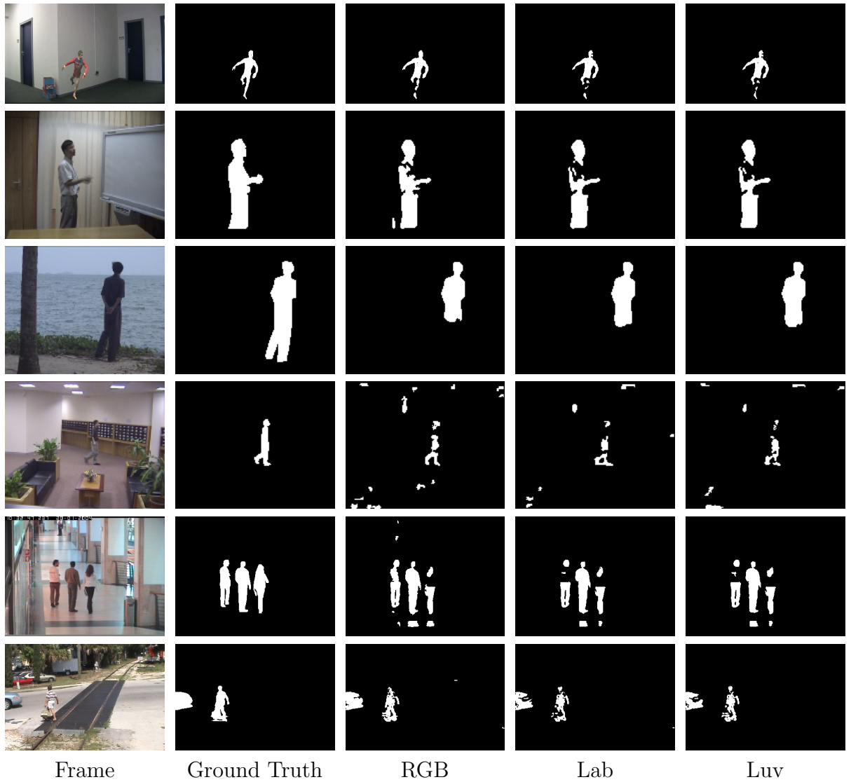
Figure 5: Foreground detection results of the GHNf model for RGB, Lab and Luv color spaces. Rows from top to bottom: Video2 (frame 526), Meeting Room (frame 23242), WaterSurface (frame 1577), Lobby (frame 2265), OneShopOneWait1cor (frame 375), and LevelCrossing (frame 386). The first two columns show the original frame and Ground Truth, respectively. The last three columns show the corresponding tested color spaces.
