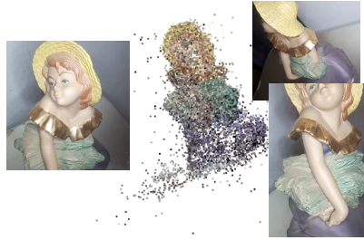
Figure 6.1: Sparse point cloud generated from a set of images.
