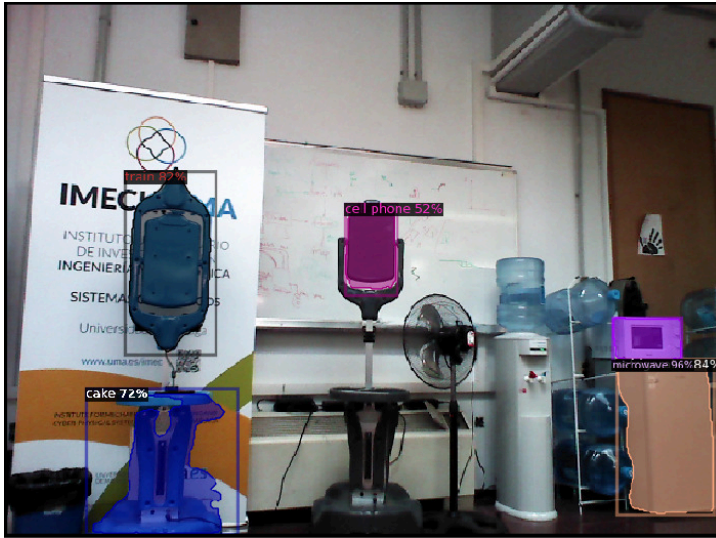
Figure 1.2: Illustrative example of the degraded performance of the Detectron2 [8] object detection network on an image containing out-of-distribution objects. The results demonstrate that the network correctly identifies in-distribution objects like the refrigerator (84%) and microwave (96%). However, it produces overconfident yet incorrect classifications when encountering out-of-distribution objects such as mobile robots, labeling them as a cake (72%), a train (82%), and a cell phone (52%).
