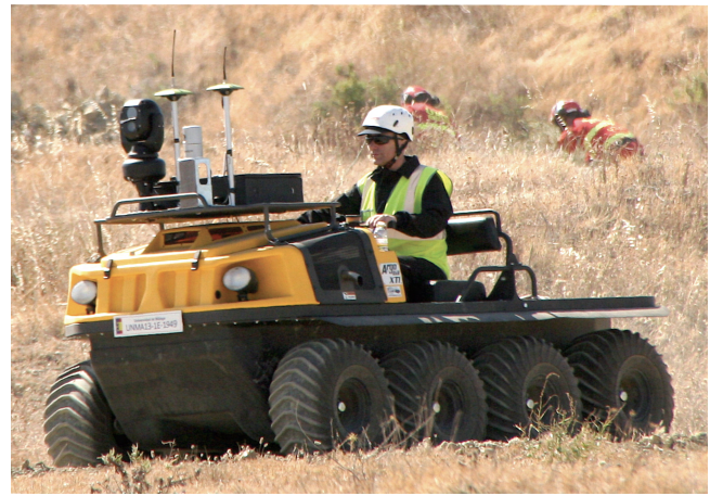
Figure 3. All-terrain Argo vehicle with the sensor suite on the front rack. The photograph was taken during the 2019 exercise.
