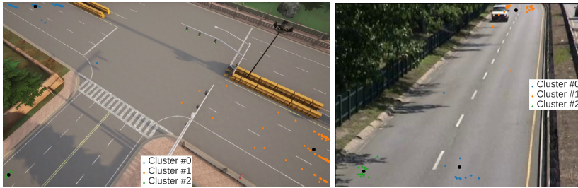
Fig. 1. The initial image frame for the first video synthesized with CARLA (left) and for the video Highway from the 2014 CDNET dataset (right). Initial/final points from each detected vehicle trajectory are drawn over the frame. Points that are grouped within the same cluster (after applying K-means) are drawn in the same color. Cluster centroids are in black. Each centroid represents an area near the border where either a whole road or an individual lane gets out of frame.
