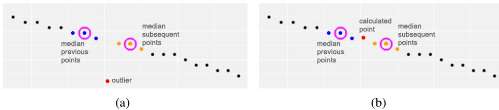
Figure 6: (a) Computation of medians after an outlier \bullet has been detected; (b) Replacement of the atypical sample using the average value of the computed medians.
