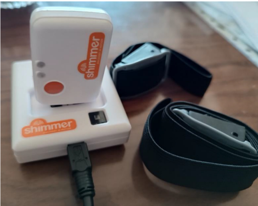
Fig. 1. Shimmer 3 node, dock station to charge the battery and retrieve the readings, snap clips and adjustable straps used to attach the sensor to the wrist.
