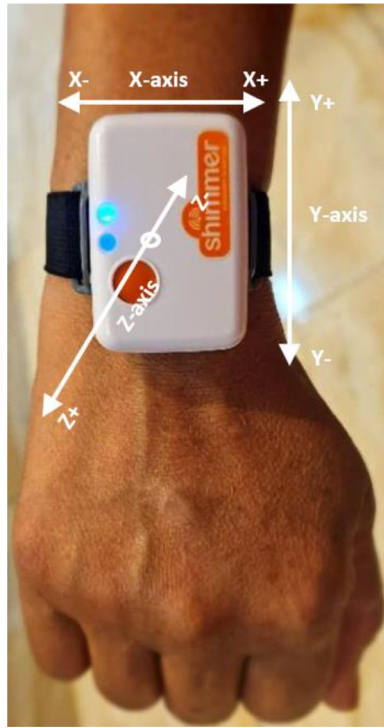
Fig. 2. Illustration of the adjustment of the sensor to the hand and orientation of the axes of the triaxial sensors.
