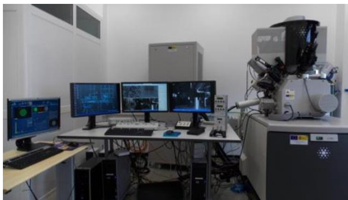
Figure 1.24. Picture of scanning electronic microscope used in this thesis, a Helios Nanolab 650 belonging to Centro de Bioinnovación y Nanotecnología of Universidad de Málaga .
