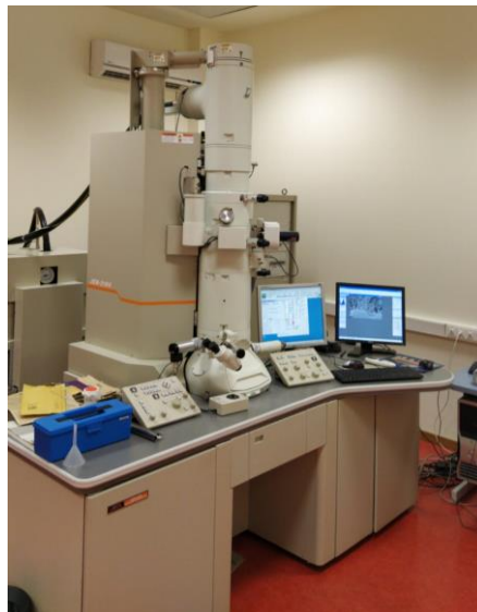
Figure 1.22. HRTEM instrument that was used for characterizing the materials belonging to the Renewable Energy Research Institute at the University of Castilla-La Mancha .
