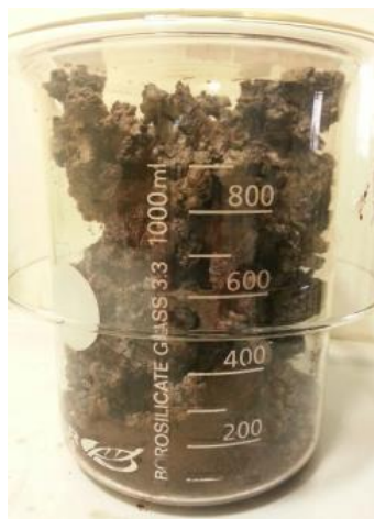
Figure 1.17. Brown powder obtained at 300\text{ }^{\circ}\text{C} 1h. This powder is ground and heated at 800\text{ }^{\circ}\text{C} 1h with a rate of 5\text{ }^{\circ}\text{C}\cdot\text{min}^{-1} to remove all organic wastes.
