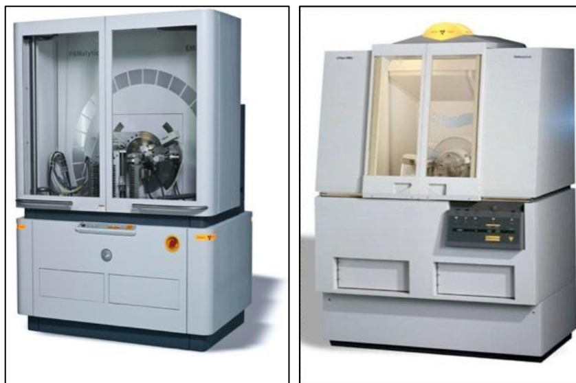
Figure 1.19. Pictures of (left) PANalytical Empyrean diffractometer and (right) PANalytical X'Pert PRO MPD diffractometer used in this thesis, belonging to the Servicios Centrales de Apoyo a la Investigación (SCAI) at the Universidad de Malaga .
