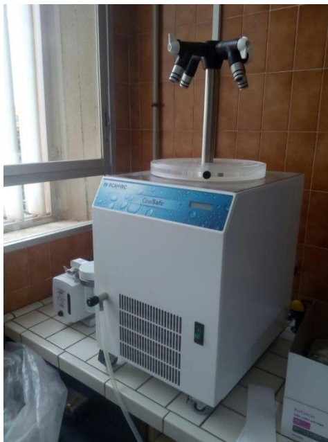
Figure 1.14. Scanvac® Coolsave™ 110-4Pro freeze-dryer used in samples preparation.
