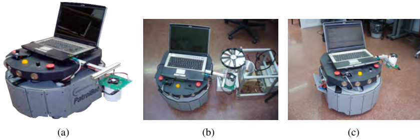
Figure A.1: Images of Rhodon at its initial stage of development. Only a laptop and a custom designed e-nose were then mounted on the Patrolbot mobile platform.
