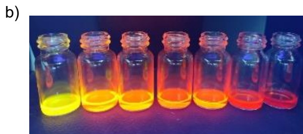
Figure 3: a) Normalized fluorescence spectra of 2d in different solvents (from left to right): 1) n -hexane, 2) toluene, 3) chloroform, 4) THF, 5) dichloromethane, 6) acetone and 7) DMF. b) Solutions of 2d in the mentioned above solvents at 10^{-5} M, excited under 365 nm light.
