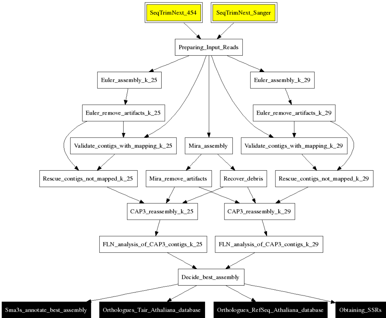
Supplementary File 1: Flow diagram of the strategy for pre-processing, assembling and annotation of the transcriptomes described in this manuscript where yellow, double-lined boxes are the inputs, and the black boxes are the output results
