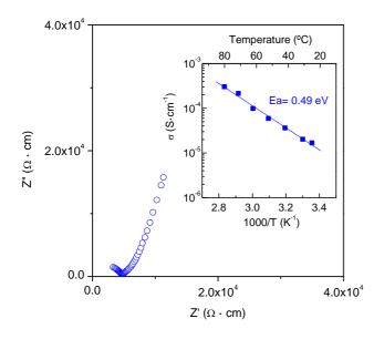
The proton conductivity of selected sample, prototype of the series, measured. In the range between and 80 ٥C. range 25° conductivity increase with the temperature up to a maximum value of 3·10<sup>-4</sup> S·cm<sup>-1</sup>, at relative humidity of 95 %. The activation obtained from energy the Arrhenius plot (Figure 1) is in the corresponding Grotthuss transfer mechanism.
