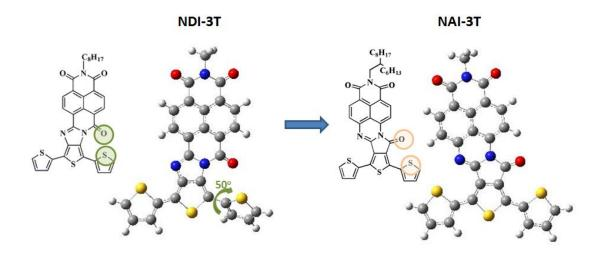
The highest FET performance is achieved for vapor-deposited films of NAI-3T with mobilities of 1.95x10<sup>-4</sup>cm<sup>2</sup>V<sup>-1</sup>s<sup>-1</sup> and 2.00x10<sup>-4</sup>cm<sup>2</sup>V<sup>-1</sup>s<sup>-1</sup> for electrons and holes, respectively. Finally, these planar semiconductors are compared with their NDI derivates analogues, which exhibit only n-type mobility, in order to understand the origin of the ambipolarity in this new series of molecular semiconductors.
