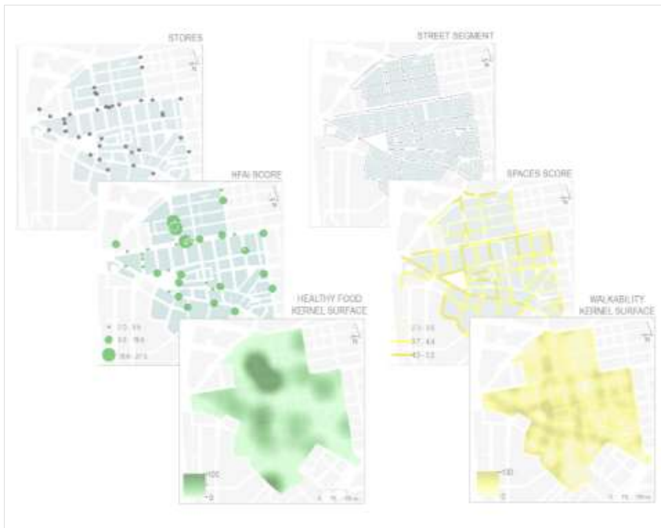
Figure 2. Development of continuous KDE variables from direct observation data. On the left, is depicts the calculating for the food environment starting with the location of all stores, continues with the Healthy Food Availability Index (HFAI) score for each one, and the next is the KDE surface weighted by HFAI score. On the right, the development for the physical activity environment. Above the location of all the street segments, continues with Pedestrian and Cycling Environment Scan (SPACES) score by each one. And in front the KDE weighted by the SPACES.
