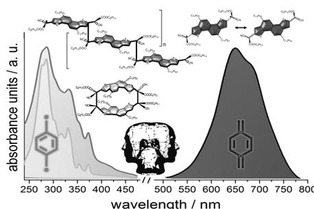
**Figure 1. UV-Vis-NIR electronic absorption spectrum of monomer and  $\sigma$ -aggregates**
