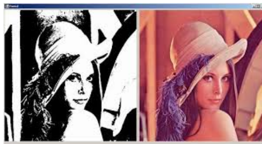
Figure 4: Thresholding technique applied on the famous image of “Lenna” comparing the original image (right) and the segmented image (left)
