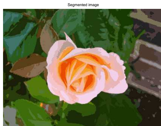
Figure 32: Figure shows the connected component images as before but having replaced the filters using a sliding window technique. In this case the parameters include a region of 7 \times 7 pixels that slides across the image replacing the pixels with the most modal pixel in that window.
