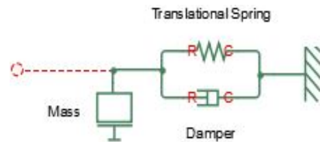
Fig. 4 SIMSCAPE modelling of the opposition to the stroke of the cylinder-piston
