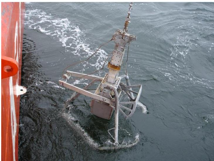
**Figura 4.4** Draga Box-Corer
