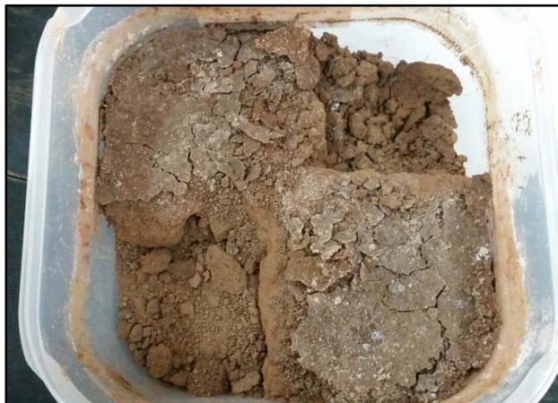
Figure S 13. Superficial precipitate observed in the superficial section of the soil stored without cover (SLC ST1)
