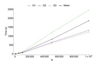
Figure 8: Quartiles and mean of the time (in seconds) required by HiReLS to find the global optimum for increasing values of N in an adjacent NKQ Landscapes with K = 2.
