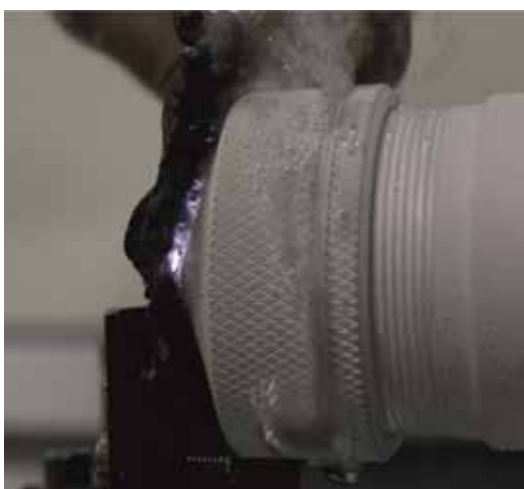
Figure 12. Laser-induced plasma during an underwater analysis of a lead sheet.
