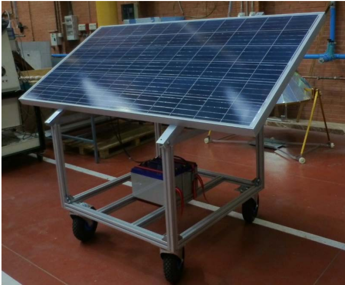
PV testing platform. Comparing using batteries is possible.
