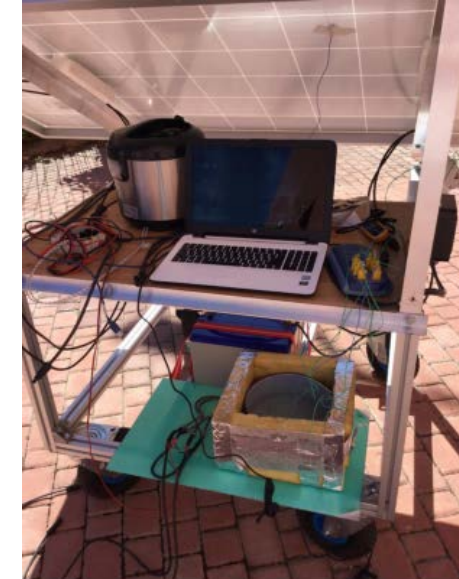
Evaporative losses experiment. Open pot on lower platform.
