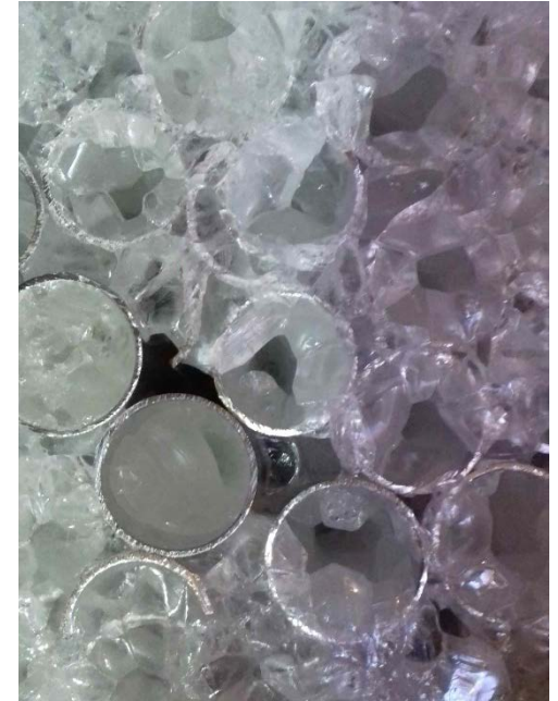
PCM retraction when solidifying.
