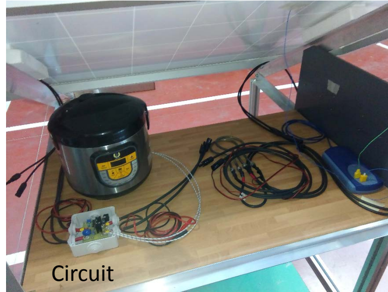
PV testing platform. Very simple PV controller circuit, pot and data logger.
