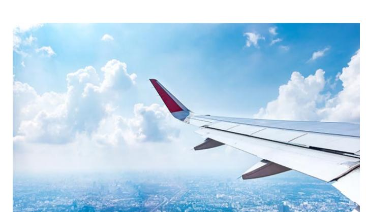
Winglets are the most widely extended solution to decrease the vortex strength.
