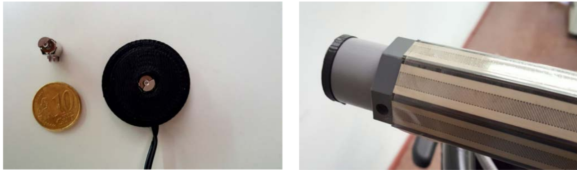
Fig. 3.49 Vibration motor and piece where it is placed (left). The whole set inserted in the left handle end (right).
