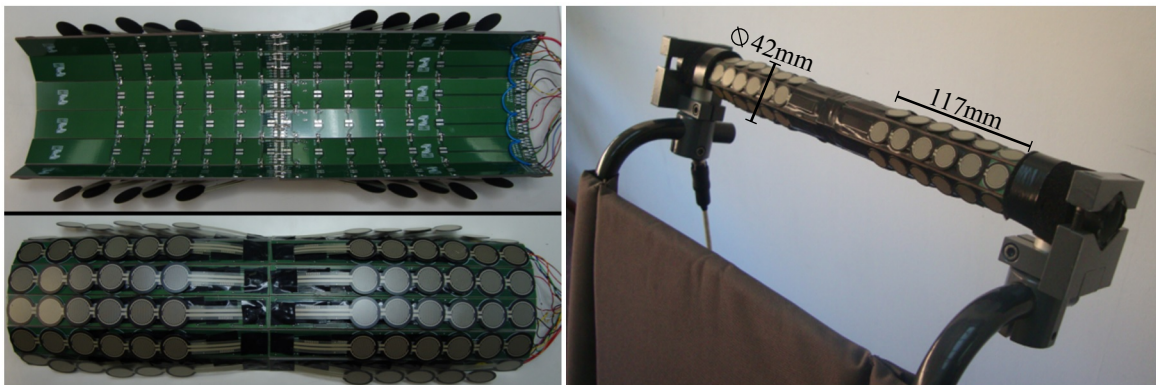
Fig. 2.7 Tactile sensors matrix prior to embrace the PVC bar (left). Resulting implementation (right).
