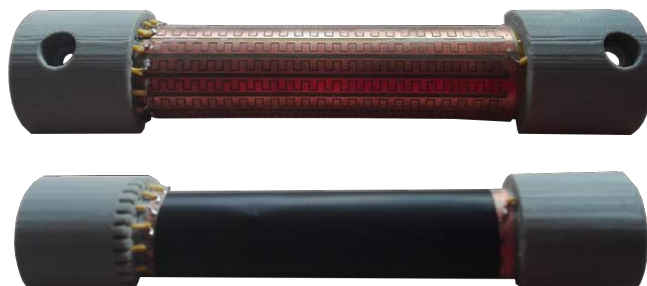
Fig. 6.2 Tactile handle equipping 16 tactels. At the bottom, the electrodes are covered with a piezoresistive sheet.
