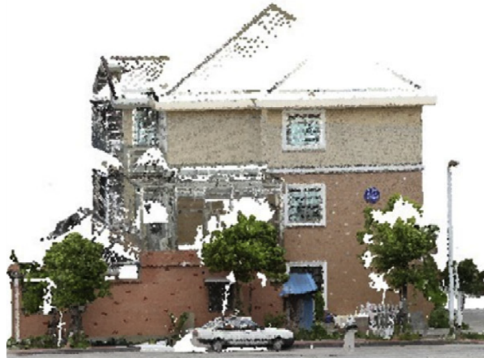
Fig. 2.3 RGB-D scene produced by combining information from a 3D scanner and a CCD camera [119]
