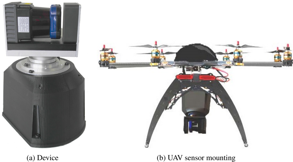
Fig. 2.7 Unomotion, a customized lidar system based on a 2D LRF in horizontal layout with a complete rotation in roll [59]. This device extends from Unolaser [63] (see Appendix A.3).
