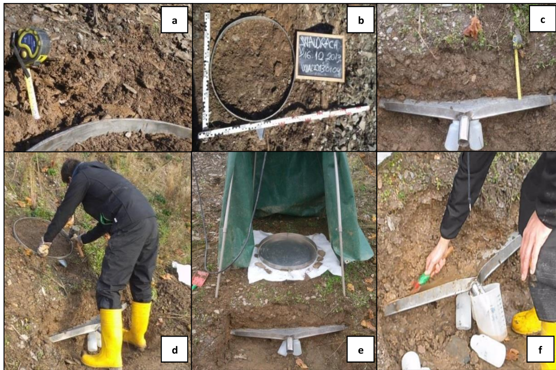
(a) A horizon eliminated (between 5 and 7 cm); (b) before simulation; (c) profile to 0.5 m below (1.5 m × 0.5 m) with the sediment collector; (d) situation of simulator ring; (e) concurrent rainfall simulation, (f) subsurface flow during the experiment.
