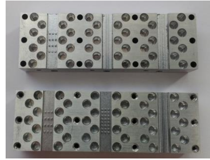
Fig. 8. Prototype manufactured that implemented both phase shifters design and the reference waveguide
