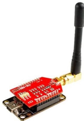
Figura 2.4. Módulo WiFi rovin networks RN-VX rev3.
