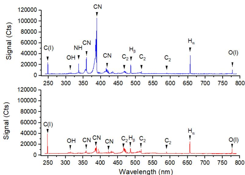
Fig.1 Ribose LIBS spectra acquired in (top panel) air atmosphere and (bottom panel) Martian atmosphere.
